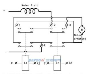
Paired Double Pole Single Throw Contactor for motor reversing. 1.2.3.4 Contact Terminal
